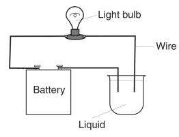
Which property of the liquid is being tested?
